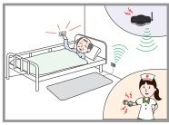
Possible to connect the system with a nurse call wirelessly when using it in a hospital. If the wandering detecting system is networked with a paging bell in a hospital room, it can be used as an emergency paging system within the hospital.
